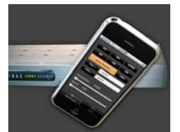
Mobile Phone steuert LINAX® Linearmotor-Achse via WiFi
